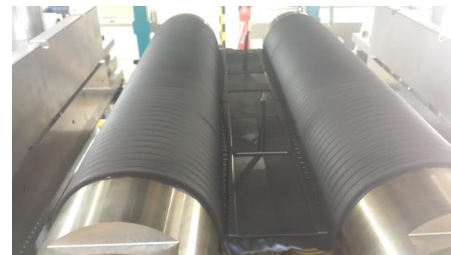
View of the seals ND110 on the core bars
