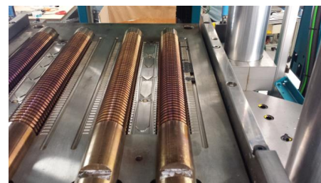
View of the 4-core mould for seals ND50
