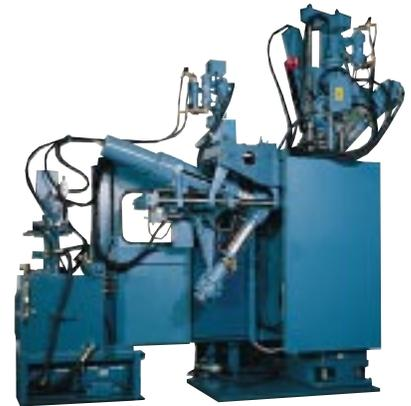
▲ *Dual-compound injection technology or how to inject two compounds sequentially or simultaneously. In either case, one compound is injected at the top while the second is injected at the mould parting line.*
