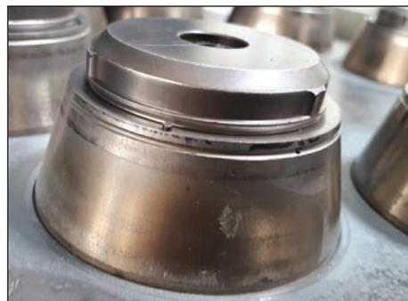
Fig. 2: Example of mold difficult to clean due to undercuts.
