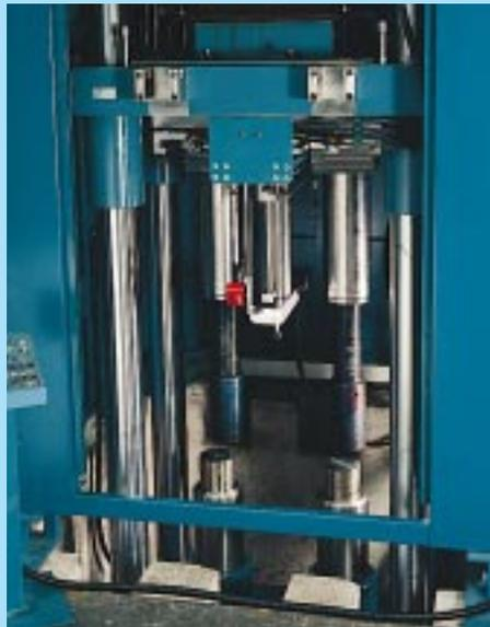
▲ Hydraulic Ejectors on Moving Traverse
