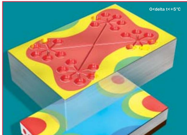
With standard heating platens, curing time has to take temperature variations into account, which often means that it is overestimated. This causes a loss of both, time and quality, and has led REP to develop the exclusive Isothermould system.
