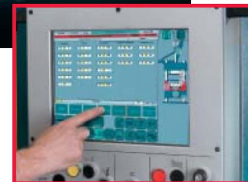
▲ Interface access levels differentiated according to the user, also protected and configurable. Different possible access modes:
