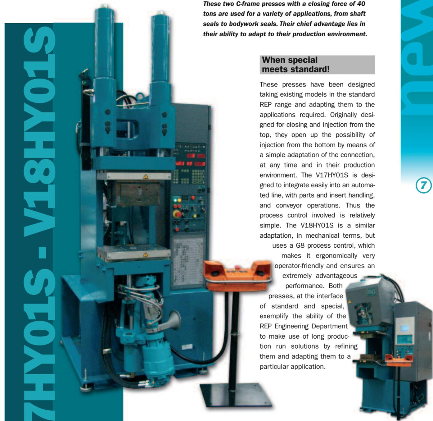
*These two C-frame presses with a closing force of 40 tons are used for a variety of applications, from shaft seals to bodywork seals. Their chief advantage lies in their ability to adapt to their production environment.*
