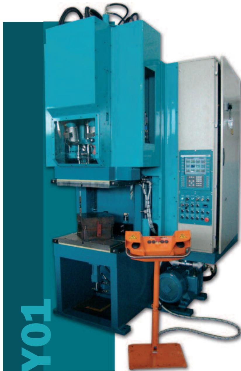
*This is a C-frame press intended for the duplicate moulding of gaskets in vehicle bodywork. It is designed to bend into the numerous configurations required by this type of production.*
